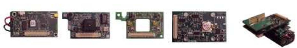
Fig. 6. Sensor hardware from left to right: (a) Mica2 network node, (b) Mica Sensor Board, (c) Mica Power Board, (d) TWR-ISM-002 Radar Board, and (e) All of the boards attached together.
