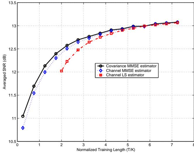
Fig. 1. Performance measure in (3) for different transmit beamforming estimators.  $M = 12$ ,  $K = 4$
