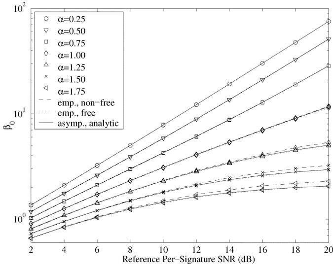
Fig. 6. Empirical and asymptotic values of  $\beta_0$ , and empirical values of  $\text{Tr}[\mathbf{R}^{-1}]$  versus per-signature SNR for a range of  $\alpha$  for two equal-power, equal-rate users.
