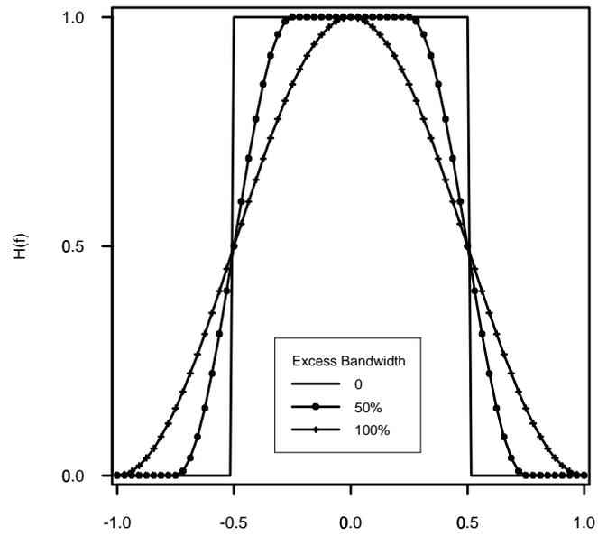
Fig. 6(b). Raised Cosine Spectrum.
