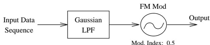
**Figure 13.** Generation of GMSK signal (LPF is Low-Pass Filter).
