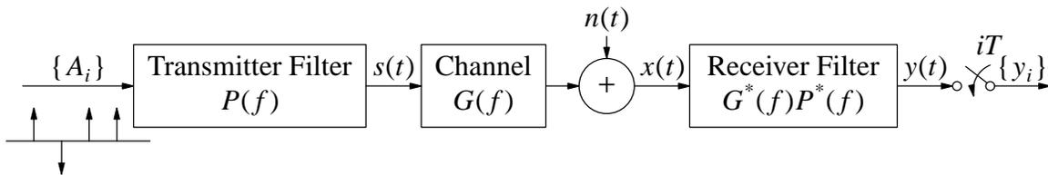
**Figure 7.** Baseband PAM model with a matched filter at the receiver.
