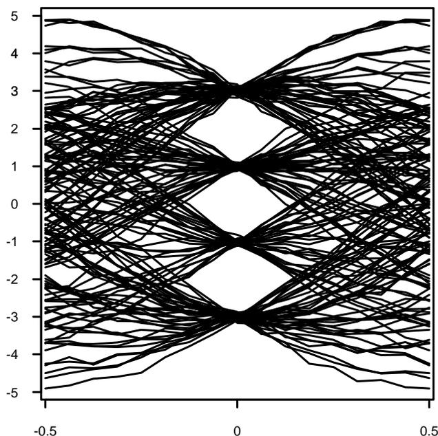
Fig. 8(b). Eye diagram for received signal shown in Fig. 8(a).
