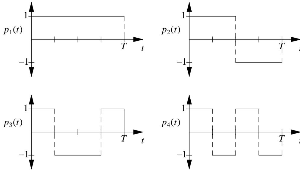
**Figure 2.** Four orthogonal spread-spectrum pulse shapes.
