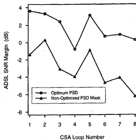
Fig. 5. Comparison of ADSL performance on all 8 CSA loops, with the proposed ADSL PSD mask (at  $-34$  dBm/Hz above 200 kHz), and the optimized ADSL transmit spectrum. The T1 margin (0.3 dB), and HDSL and ISDN BRA margins (approximately 12 dB or more), are the same for both transmit signals. Data rate is 6.536 Mb/s.
