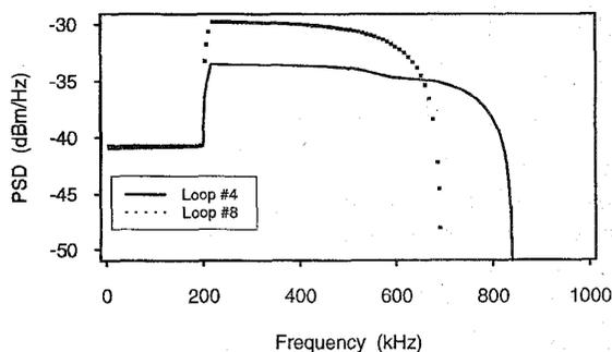
Fig. 2. Example of the line dependent, optimized ADSL transmit power PSD's for CSA loops #4 and #8. Optimized PSD's for the other 6 CSA loops fall within these two bounds.
