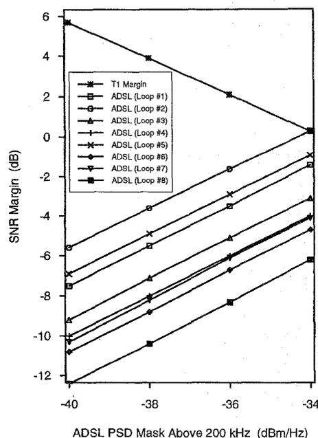
Fig. 3. T1 and ADSL performance margins as a function of the proposed ADSL PSD mask in [9]. Below 200 kHz the PSD mask is fixed at  $-40$  dBm/Hz. In all cases, the nominal HDSL and ISDN BRA performance margins are approximately 12 dB or more, on all 8 CSA loops. Data rate is 6.536 Mb/s.
