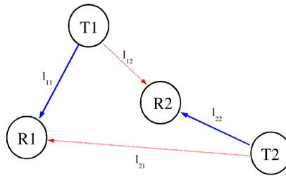
Fig. 3. Simulation scenario in which the location of the transmitter T1 is uniformly distributed within a circle centered at R2, and R1 and T2 are placed at random locations within circles centered at T1 and R2, respectively. ( $l_{11} \leq d_0$ ,  $l_{22} \leq d_0$  and  $l_{12} \leq d_0$ )
