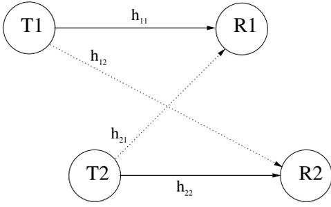
Fig. 1. Interference channel with two transmitter-receiver pairs
