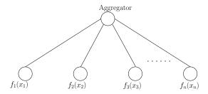
Fig. 1. Parallel architecture to implement the proposed algorithm.
