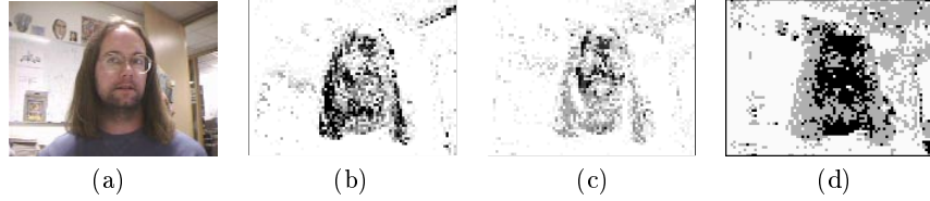
Fig. 7. (a) A raw image, as input to the final tracking function. (b-c) likelihood of pixel skin-color, based on learned final model (likelihoods scaled so that highest is darkest), with total weight of training data size kept constant: (b) 1 sample from each frame; (c) data weighted by ellipse residual (1 sample from each frame, for 70% of frames). (d) Bayesian decision to separate foreground from background: Black pixels mark foreground pixels; gray pixels mark potential foreground pixels which are more likely to be background.
