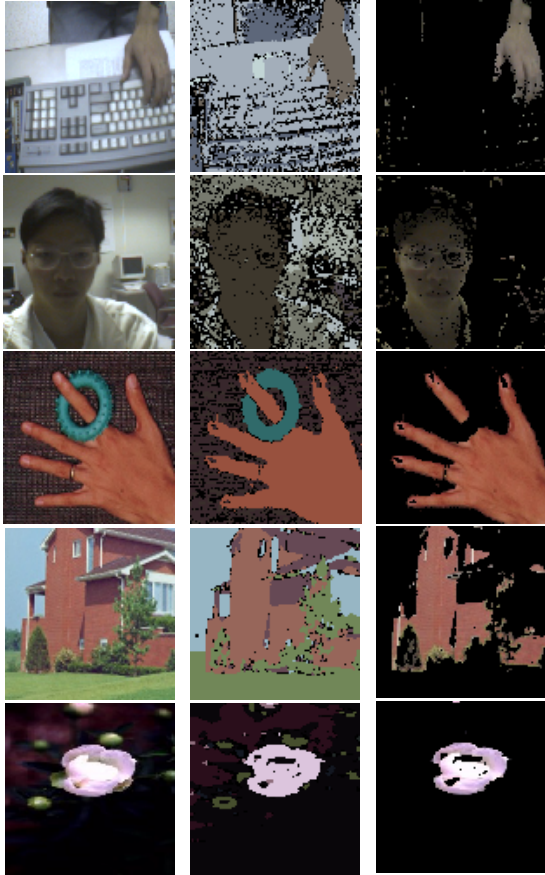
Figure 4. Color segmentation results. Left column are source color images, middle column are segmented images and right column are interested color regions.
