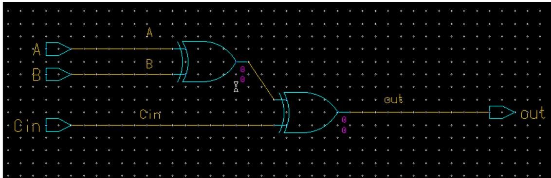
7. Now we should save our work. File->Save Sheet. We then Check->Sheet and Check->Schematic to see if we have any problems. A warning in Check schematic is expected regarding no pins in the interface.
