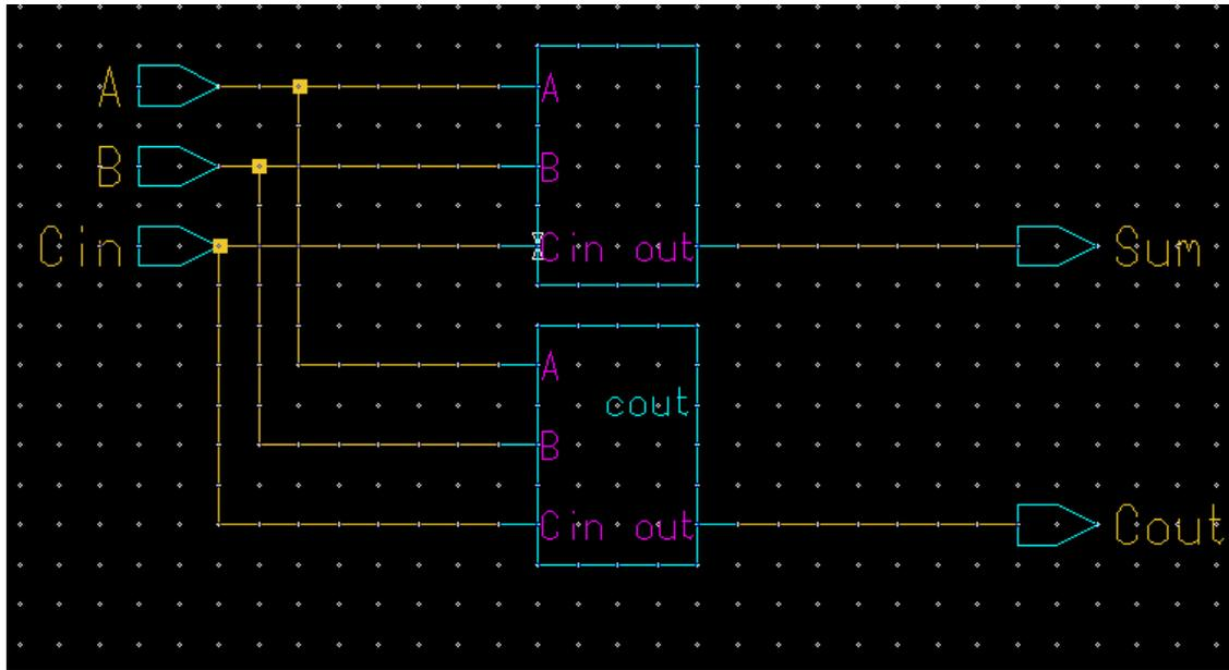
12. Now Check->Sheet and Check->Schematic before saving. Generate a symbol as we did in the past. Make sure to do all the proper checks after generating and saving a symbol and also after creating the symbol for the schematic. Close everything in design architect and then close design architect.
