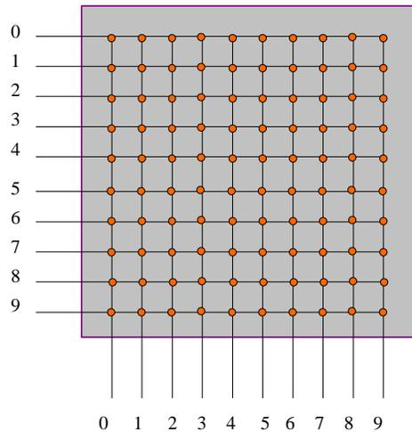
**Space Division switches** Crossbars are somewhat inefficient and require large number of cross-points. (The number of crosspoints is a measure of the complexity of the switch.) A more efficient design is to use several smaller crossbar switches and interconnect them. The resulting switch is called a **(multi-stage) space division switch**. An example is shown next.
