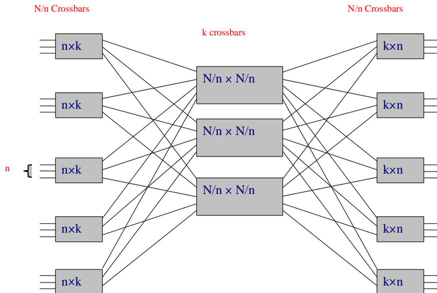
Suppose there are  $N$  incoming and outgoing ports. These are divided into  $N/n$  groups of  $n$  ports. Each group of  $n$  incoming ports is attached to a  $n \times k$  first stage crossbar switch. The  $k$  output ports of each of these switches are connected to one of  $k$  second stage  $N/n \times N/n$  switches. Finally there is a last stage of  $N/n$   $k \times n$  switches. An incoming call is switched through all 3 stages.
