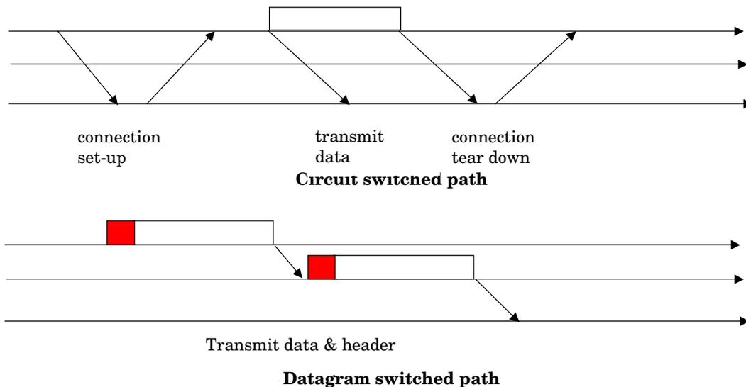
These timing diagrams show a single packet sent on a circuit switched network and a datagram switched network. Here we assume that in both cases the entire transmission rate is used for the packet. In the circuit switched case, if FDM or TDM is used, then the transmission time would be longer. For the circuit switched approach, extra delay is incurred for call set-
