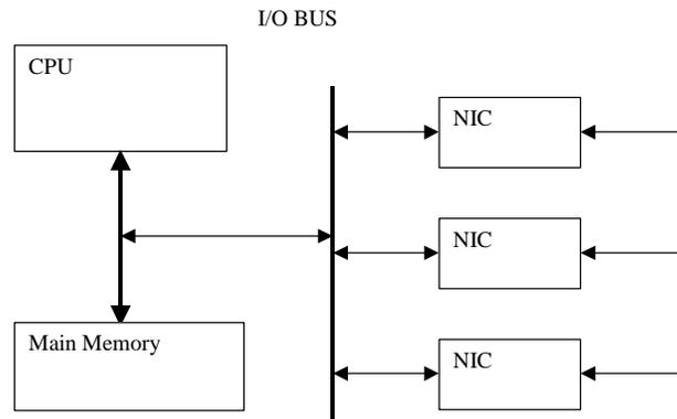
In this switch, when a packet arrives, it gets transferred into memory. The CPU executes a routing table lookup for output port. The packet then gets transferred to the output NIC and forwarded. In this buffering is needed in the interfaces for each input, in case the I/O bus is busy. This design can be limited by the I/O bus speed, the memory bandwidth, or the CPU speed.
