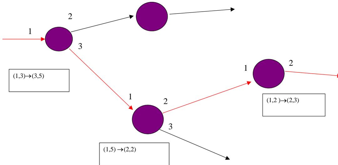
Each box shows the forwarding table entry for a connection along the path shown in red. The notation used is (incoming port, VCI) → (outgoing port, VCI). Thus at the first switch, packets arriving with VCI 1, will be forwarded to port 3 and their VCI will be set to 5.
