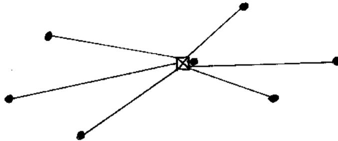
This now requires only  $N$  links and one switch with  $2N$  ports. Now, if each user only sends traffic to one other user at any given time, then multiplexing is needed on the links outgoing from the switch (or some users may be **blocked**)
