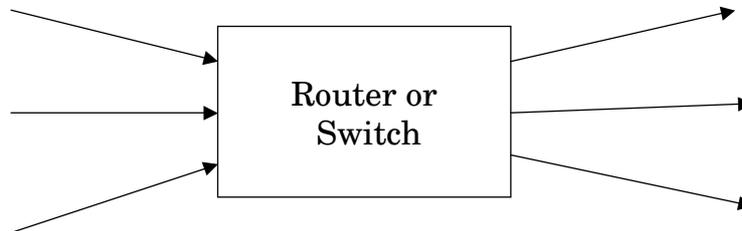
The transmission links in subnet usually carry traffic from several users. How this traffic is combined onto a link is referred to as **Multiplexing**.
