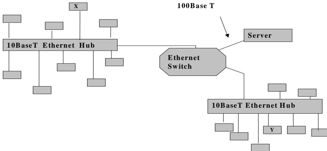
Packet from X->Y must contend with other nodes on left Ethernet LAN, to be received by the switch. The switch then contends to transmit packet on the right LAN.
