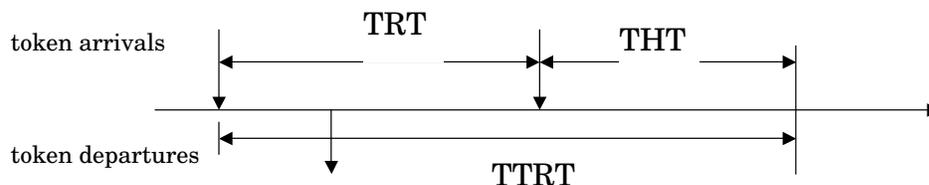
Suppose a station transmits for a long time before releasing its token by sending a lot of asynchronous traffic. The next time the token arrives, its THT will be small, and will not be able to send much asynchronous traffic.
