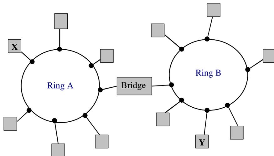
For X -> Y packet, bridge must receive packet from ring A and acknowledge packet, acquire token on ring B, and forward packet to Y.
