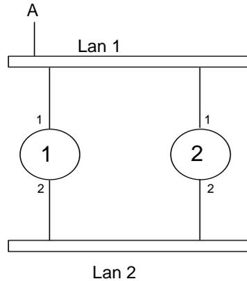
Suppose **node A** sends a packet with a destination address that is not in either bridges forwarding table. In this case, both bridges would forward to LAN 2. Each packet arrives at other bridge on LAN 2 and is forwarded to LAN 1, etc.
