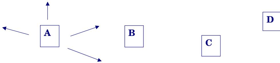
**Exposed terminal problem** - Assume B is transmitting to A and C wants to transmit to D. Here C hears B, but could transmit anyway because this would not interfere at A.
