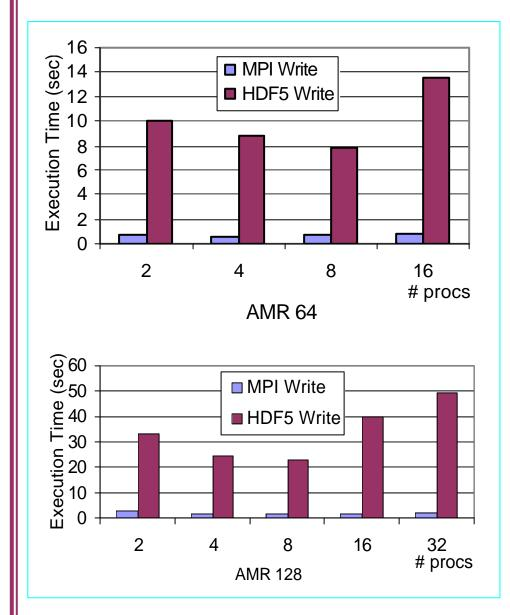
Comparison of I/O write performance for HDF5 I/O vs MPI-IO (on SGI Origin2000)
