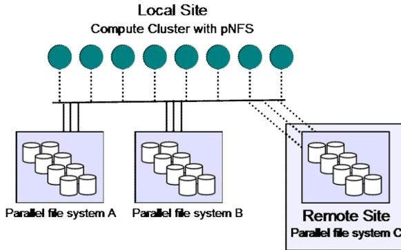
**Figure 1. Using pNFS in a compute cluster.** Applications can use a single pNFS client to mount and access their preferred parallel file system. The mounted file systems can be within the same site or across the WAN. Each compute node runs a stock Linux kernel.
