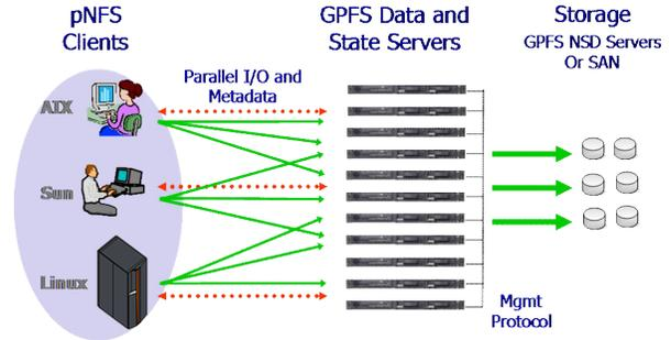
**Figure 2. pNFS-GPFS Architecture.** GPFS servers are divided into overlapping groups of state servers and data servers. pNFS clients access state servers for metadata operations and perform parallel I/O to the data servers.
